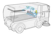
**Easy Clean System** The operator simply activates the EasyClean self-cleaning function. The blower, filter screen, dirty water tank, side walls and other difficult to reach pockets of dirt are then sprayed by the cleaning nozzles. The machine is perfectly clean within a couple of minutes.
