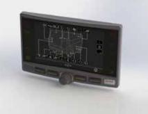
Large 7-inch central display Thanks to the diagnostics system, the 7-inch central display provides easy access to all relevant machine data such as total running time and working hours, operational and road travel, fuel consumption etc.
